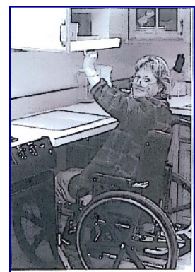
Wheelchair space under counter and stove with controls in front
